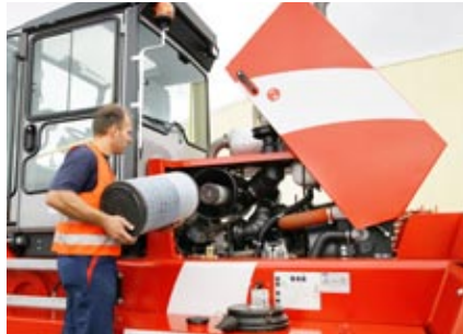
The air filter is easy accessible under the hood.
