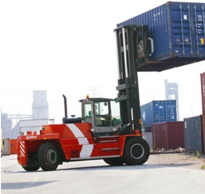
Handling of loaded 20' containers with forks.
