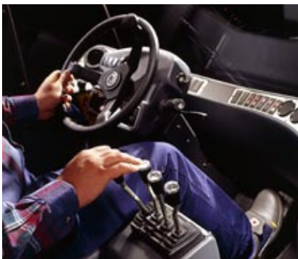
Hydraulic or electric servo control by levers.
