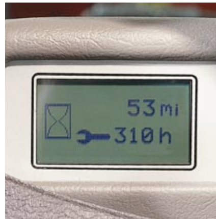
Distance since last service and hours to next service.
