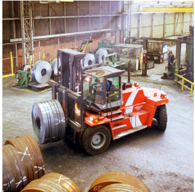
DCD240-6LB with coil ram in steel operation.
